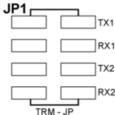
Figure 10-1: Jumper JP1 Default Locations
